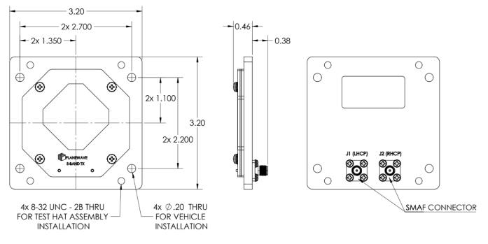
Dimensions shown in inches. Tolerances - Two Place Decimal: ±0.010, Three Place Decimal: ±0.005
