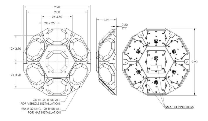
**Dimensions shown in inches.** Tolerances - Two Place Decimal: ±0.010, Three Place Decimal: ±0.005
